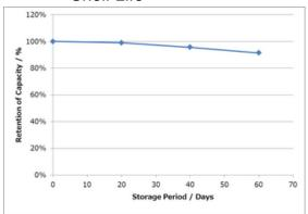
Measurement conditions:Temp:23 deg C Storage conditions: 60 deg C Dry Load: $20k\Omega$
